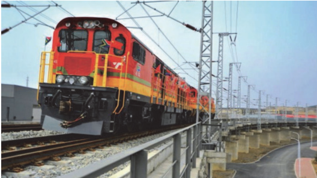
Figure 1-4 A CRRC 45D diesel locomotive running on the railway in South Africa
